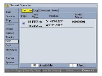
When the GPSMAP 2106/2110 is connected to a VHF radio with DSC support, the GPS unit displays a call list, log, and a directory that stores incoming information received from another user's DSC-capable VHF/GPS combination. Basic wiring is required for the Garmin unit and VHF radio to send and receive NMEA data from each other. See the *GPSMAP 2106/2110 & GPS 17 Installation Instructions* for more information.
